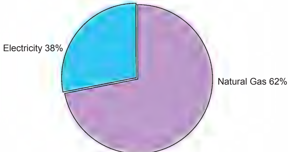
Figure 39. Weighted Average Breakdown of Dollars Spent per Year on Natural Gas and Electricity in NFDM Plants
