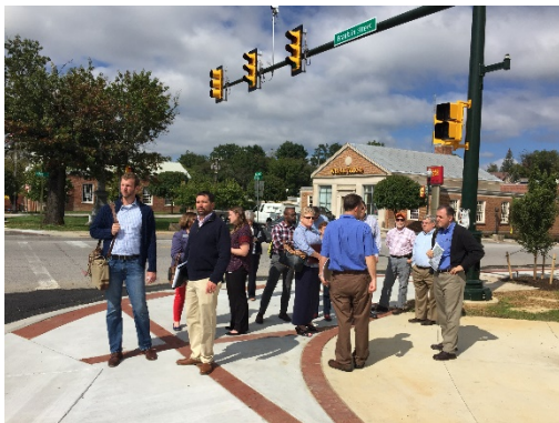
Figure 2 - The town has rebuilt its sidewalks downtown and used curb extensions to shorten crossing distances. This has improved the walkability of the area. Image Credit: Mike Callahan, Renaissance Planning.
